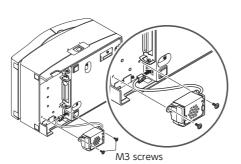
2. Pull the 4 hooks on the lower case outwards, and remove the upper case. Remove the 2 screws, and remove the buzzer from the lower case. [See Fig. 1]
